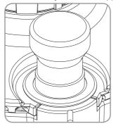
To ad just the number of grams in a single dose, use the dial (7) on the bottom part of the doser (9), turning it clockwise to increase the size of the dose and anticlockwise to reduce it.
